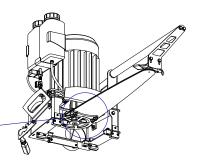
Correct chain tension: If you hold the chain between your thumb and forefinger, you should be able to pull the chain out from its groove at the middle point of the bar. When releasing the chain it should snap back into the groove in the bar. A new chain slackens quickly. Tighten a new chain after the first and the second saw cut.
