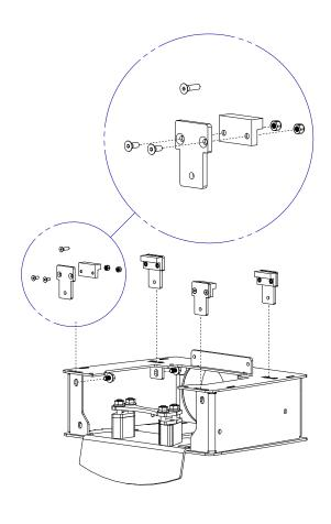
3. Press the eight M4 lock nuts into the vertical guides (20). Use the supplied M4x16 countersunk Allen bolt. Use the foot plate (19) as a counterhold. At the start, the nut has to be held by a 7 mm combination spanner in order not to rotate. Tighten until the nut fully touches the bottom. Then, unscrew the bolt and replace it with a M4x8 countersunk Allen bolt, as in the illustration.
