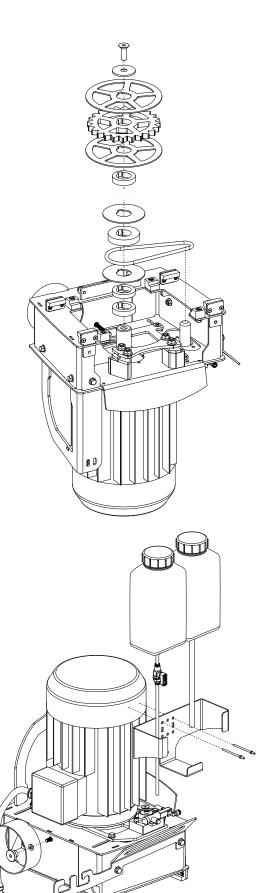
7. Turn the machine upside down and install the following components on the motor shaft in this order: two 10 mm spacers (32), belt guide (33) and oil pump sheave (34). Then, fit the round belt (35) between the sheave and the oil pump shaft (44).
