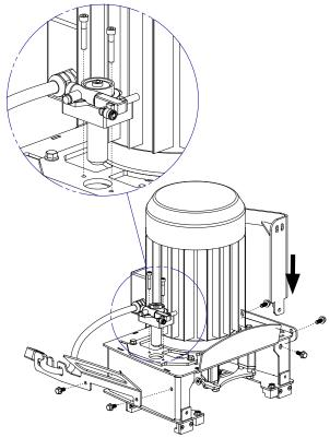
6. Turn the saw unit around, so that it stands on its "feet".
