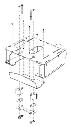
2. Fit the sawdust guard (7) to the chassis (3). Use five M4x8 countersunk Allen bolts. Then, install the guide bar spacers (11) and the guide bar plates (13) using four M8x65 countersunk Allen bolts. Tighten the bolts firmly. Install the cover plate (14) and thread four M8 flange nuts (Tensilok) onto the ends of the Allen bolts. Leave a 5 mm play between the guide bar plates and the cover plate, so that the guide bar (12) easily can be installed later.
