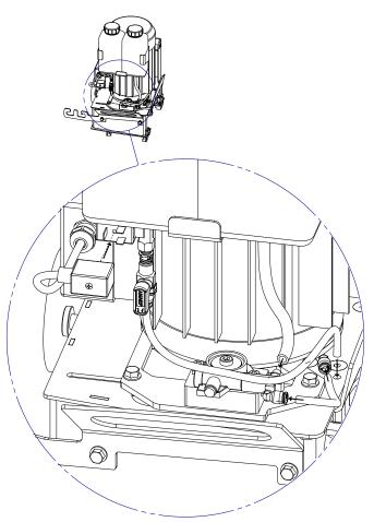
9. Connect the rubber tube (22) from the oil bottle (28) to the inlet of the oil pump (37). Secure the tube to the oil pump inlet with a tube clamp (45).
