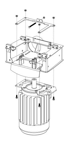
5. Place the chassis (3) on the motor mount (8) as in the illustration. Install a fully threaded M6x75 hex bolt in the chain tensioner (9) and fasten it with an M6 nut, as in the illustration.
