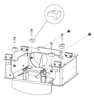
4. Fit the four horizontal guide blocks (21) to the chassis (3). Use M6x20 Allen bolts and M6 flange nuts.
