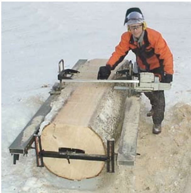
Big Mill PRO: LSG with double guide rails, Arm EXT and Fixing Plate EXT. The slide profiles (no.4 page 27) do not touch the log.
