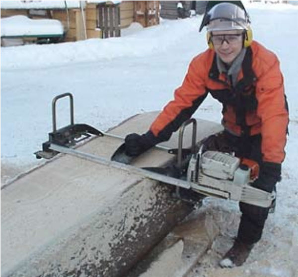
LSG without guide rails. The plane surface of the log steers the next cut.
