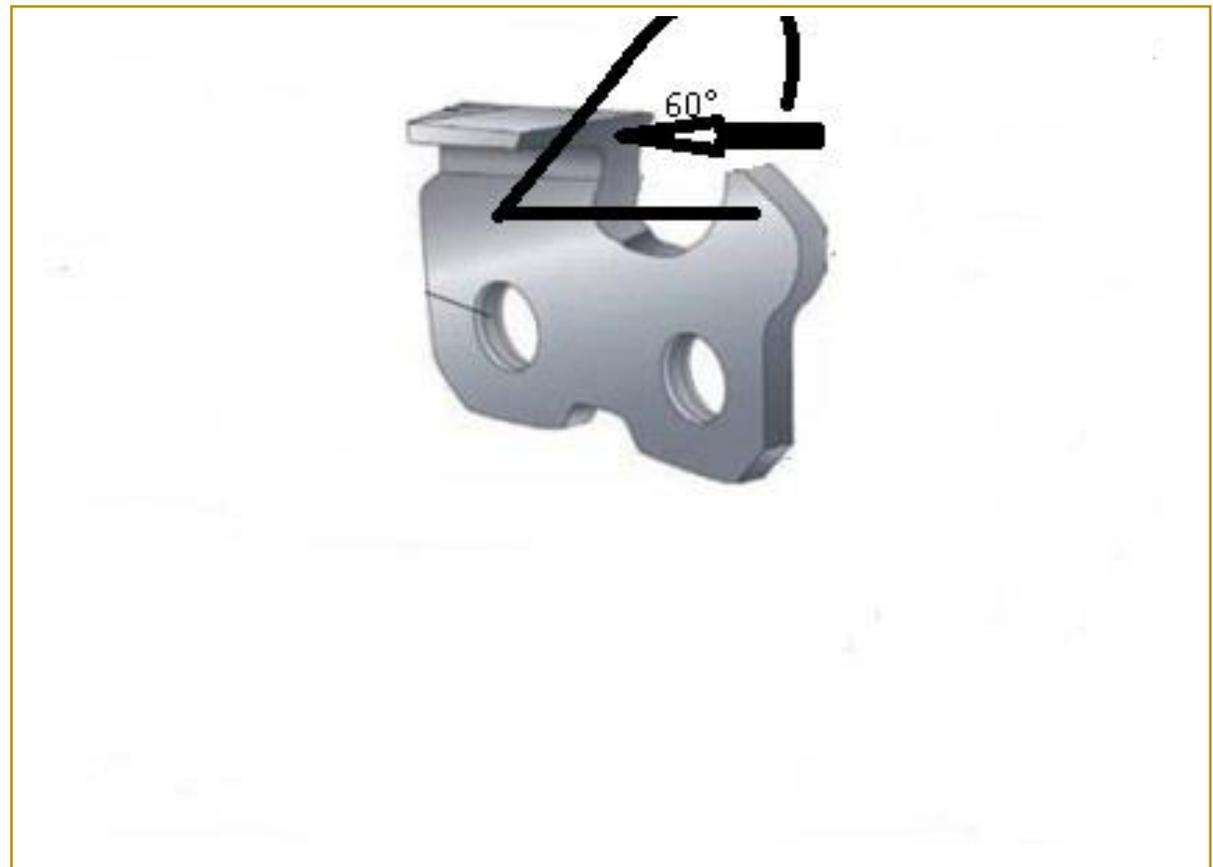
Make sure that you have the right chain sprocket. A PMX/RMX chain (low profile chains) fits on a standard 3/8 sprocket, but you cannot use a standard 3/8" chain on a Picco sprocket. If you do that the drive links of the chain will get deformed, which leads to heat building up and, ultimately, the chain will get wedged between the bar rails.
