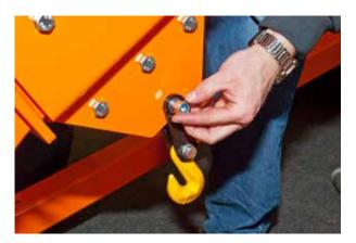
11. Fit the link plates and the lifting hook to the slliding rail, using **two M10x40** including **M10 lock nuts** and **M10 washers**.
