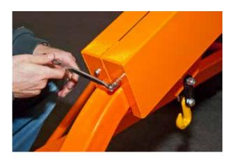
12. Fit the cover over the sliding rail with the opening for the tube arch facing the rear of the trailer. Secure the cover with **four M6x16** including **M6 washers**.
