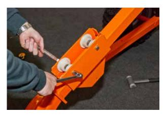
Assemble the side pieces, including rollers, using two M10x100, two M10 lock nuts, two M10 washers and three M10x25, three M10 lock nuts and three M10 brickor.
