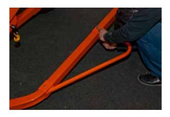
13. Fit the wheel guards on each side of the frame, as seen in the picture. Use **four M8x80** including **M8 lock nuts** with **M8 washers** on the side where the nuts are.
