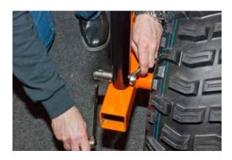
7. Secure the tube arch with two M10x60 + M10 lock nuts and M10 washers.
