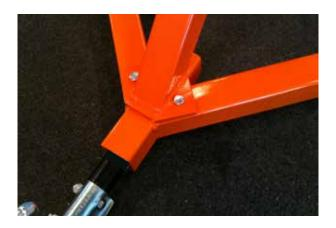
Fit the sliding rail front mount to the frame using two M10x85 + M10 lock nuts and M10 washers on the side where the nuts is.
