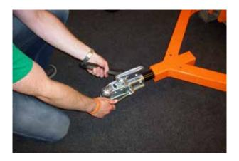
Install the black tube spacer on the trailer hitch axle and then fit the ball coupling using two M10x55 + M10 lock nuts.
