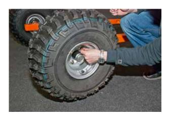
5. Fit the wheels using the included **M12 wheel nuts**. Note that the tapered side of the nut should be facing the wheel rim, in order to centre the wheel on the hub.
