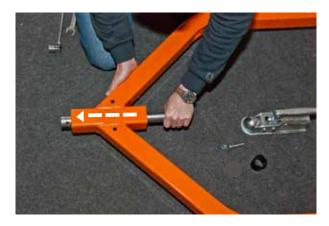
2. Insert the trailer hitch axle, as seen in the picture.
