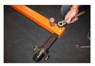
4. Fit the wheel hubs by inserting them into the square-shaped holes at the rear of the frame, as seen in the picture. Secure them with one M12x60 + M12 washer and one M12 lock nut (the nut is placed in a hexagonal hole on the lower side of frame). Tighten firmly.
