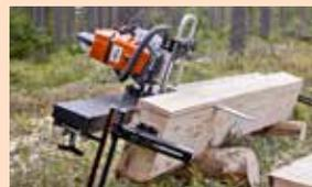
When three sides of the log are cut, you can start sawing your planks and boards. The rail acts as a guide for the first cuts.
