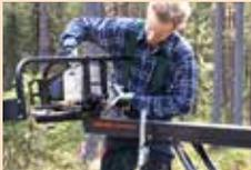
The chainsaw is easily mounted on the carriage, which slides smoothly and accurately on the guide rail.
