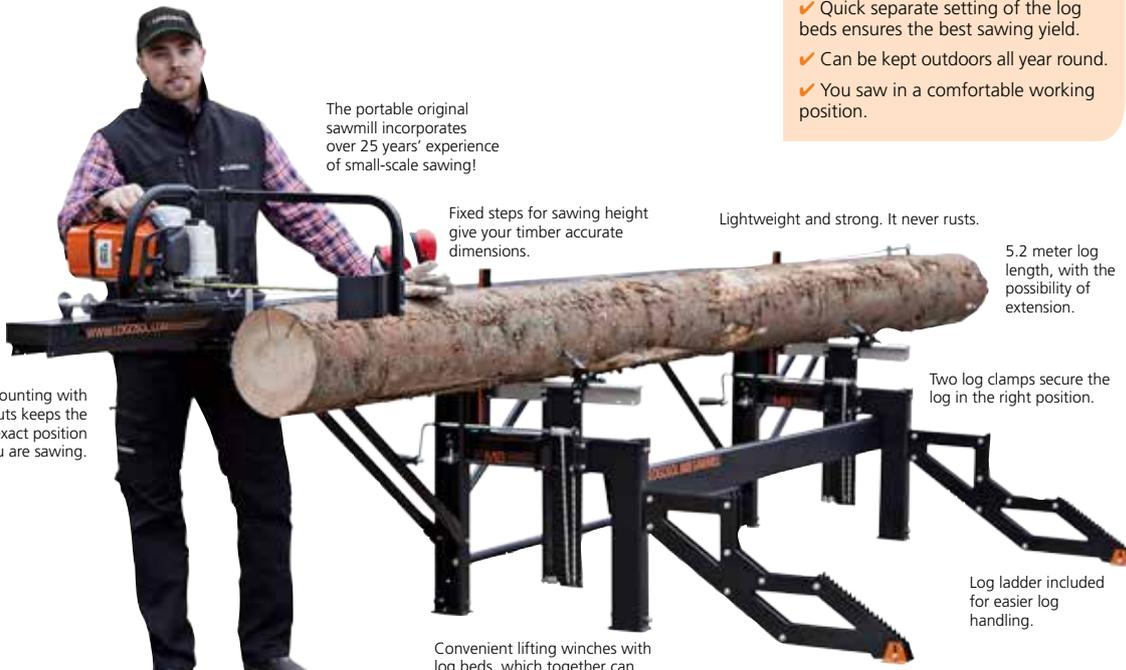
The portable original sawmill incorporates over 25 years' experience of small-scale sawing!
