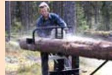
The first cut! The log is secured, and you saw by cranking the carriage forward.
