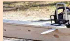
After that, the guide rail is removed and you cut the boards using the Timberjig directly on the cant. The board thickness is set with stepless adjustment.
