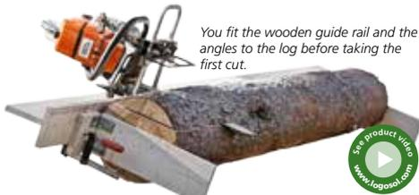
You fit the wooden guide rail and the angles to the log before taking the first cut.
