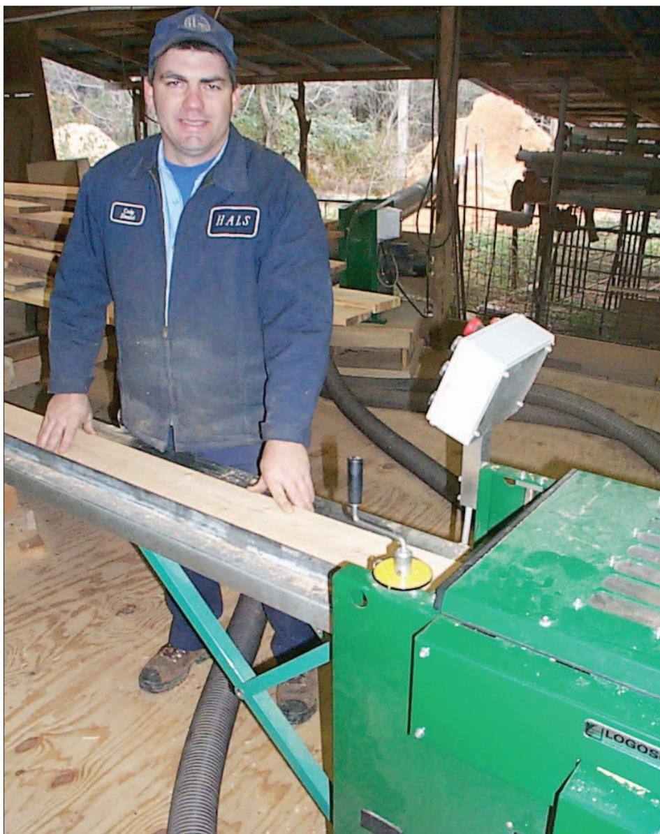
*Craig Howard with Logosol PH260 Planer-Moulder; the machine is fitted with a chip extractor also made by Logosol.*
