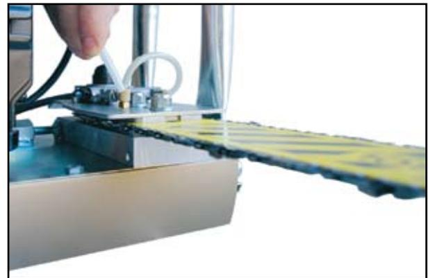
*The white plastic tube is pressed down into the drilled hole, and stays there due to the hole being narrow for the tube.*
