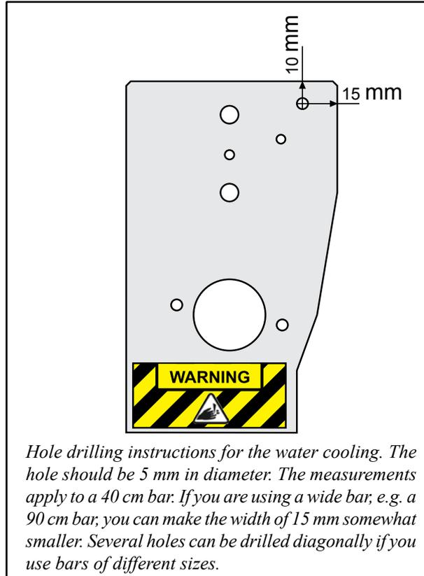
*Hole drilling instructions for the water cooling. The hole should be 5 mm in diameter. The measurements apply to a 40 cm bar. If you are using a wide bar, e.g. a 90 cm bar, you can make the width of 15 mm somewhat smaller. Several holes can be drilled diagonally if you use bars of different sizes.*
