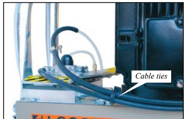
*The bar attachment seen from the back. Ensure that tubes and cables are fitted so that they do not run the risk of getting caught in something during operation. Also consider that the tubes should be of a length that does not make it difficult to replace the chain. A good solution is to fasten the tubes together using cable ties, as on the picture above.*
