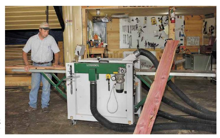
Rusty with his PH260 Model 3. Notice the setup tools attached to the front of the planer on a magnetic strip. The kiln Rusty built is behind him.
