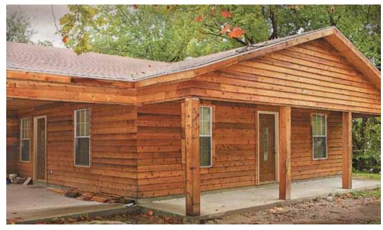
Rusty produced all the wood for this house from reclaimed fir. The siding was run on the Logosol PH260, as well as the interior paneling, mouldings, and wainscoating.
